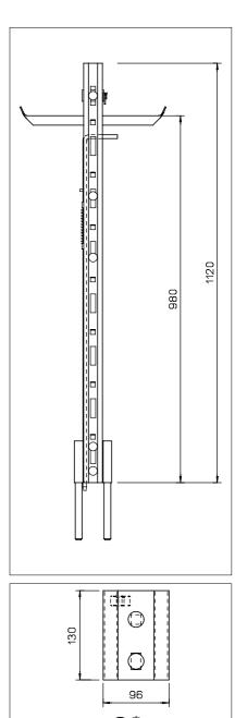
This device is fixed to the top of the guide-rail in the manhole. Stainless steel, pickled
